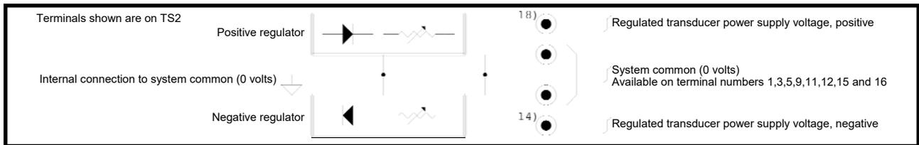
The connections shown above are included for user's who plan to use the dancer position regulators internal power supplies to drive external feedback or command transducers in addition to or in place of the normal position command and feedback potentiometers.
