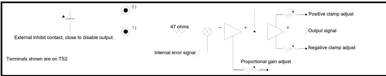
The external inhibit contact is used to force the output signal from the dancer position regulator to zero. When the inhibit contact is closed the output of the dancer position regulator will be clamped to a value of less than .050 volts. The current flow through the inhibit contact is internally limited to a maximum of 10 ma., accordingly this contact should be rated for low level or dry circuit switching operation.
