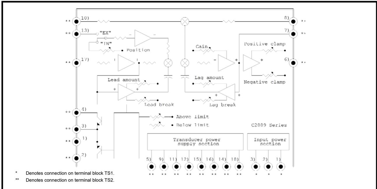
The functional drawing in the figure above illustrates the signal flow and polarity as well as the interconnections between the signal processing modules supplied on the dancer position regulator circuit board assembly.
