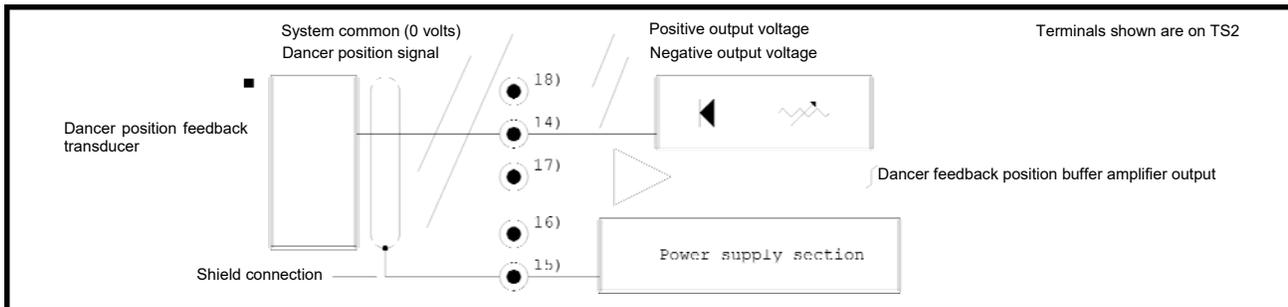
The figure above shows the connections between the dancer position regulator and a external dancer roll position feedback transducer. The dancer roll position feedback transducer must be connected to the dancer roll assembly so that full travel or loading of the dancer roll does not cause the output from the transducer to exceed the rated input signal to the dancer position regulator.
