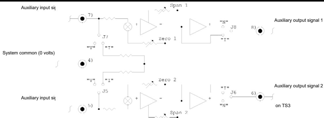
Both of the scale sections will accept either voltage or current input signals. The type of input signal is determined by the position of jumpers "J5" and "J7". With either of these jumpers set to the "V" position, the input signal to the associated amplifier should be obtained from a voltage source. When the associated jumper is in the "I" position the input signal should be obtained from a current source.
