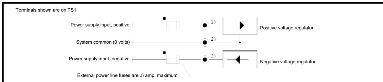
The fuses shown in the connections to terminal numbers 1 and 3 on TS1 are not required if the user's external power supply includes the necessary short circuit protection devices.
