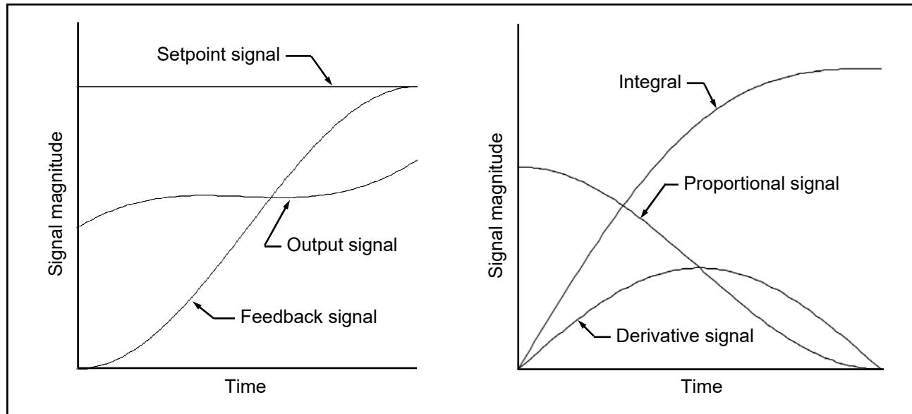
The graphs in the figure above illustrate the relationship between the controller signals in response to a step change in the setpoint value. In this example, the controller is tuned to produce a smooth response with zero overshoot.
