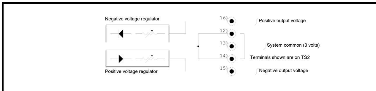
The transducer power supply output current is limited by the regulators ability to dissipate heat as well as the maximum power rating for the transformer on AC line powered models. The maximum output current at all ambient temperatures can be determined from the formula given below:
