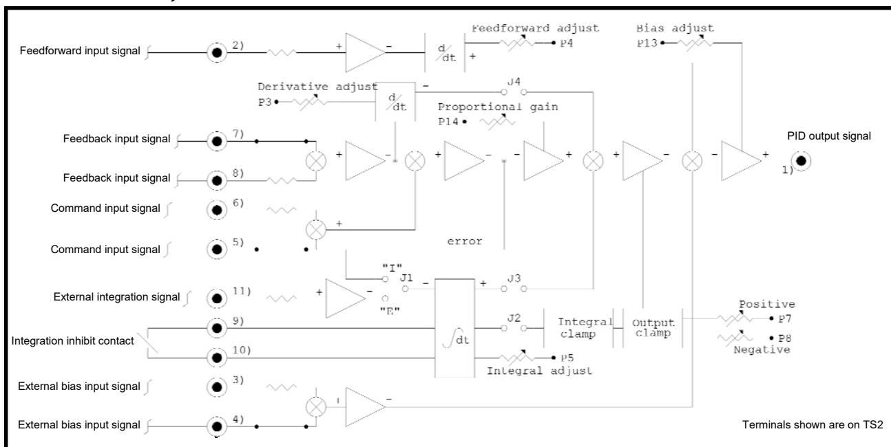
User signals applied to terminal numbers 4, 5 and 7 require that the user supply external resistance in series with these signals. The correct resistance value is determined by the maximum value of the input signal and the rated input of the controller. The required resistor value can be determined with the formula below.
