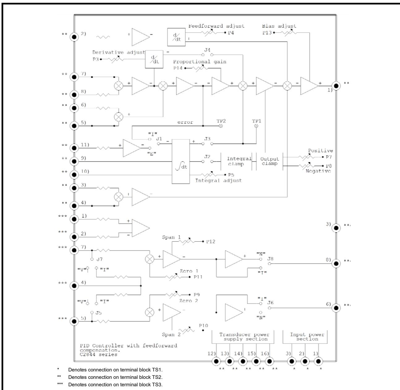
The functional drawing above shows the interconnection, signal polarities and function of the PID control and auxiliary modules supplied on the circuit board. The function and signals applied to each terminal are detailed in the chart on the next page of this manual.
