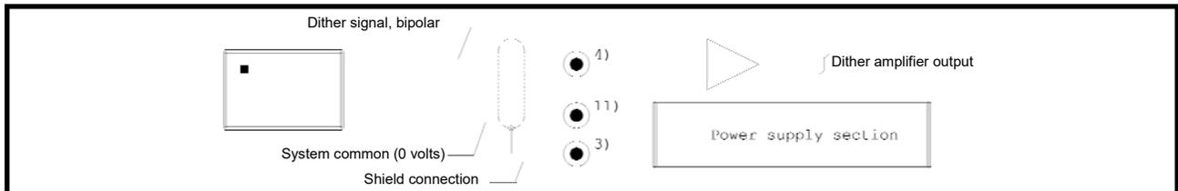
The addition of a dither signal as shown above will generally improve the hydrostatic drive's regulation and response time. The magnitude and frequency of the optional dither signal should be obtained from the pump displacement controller manufactures data sheet.
