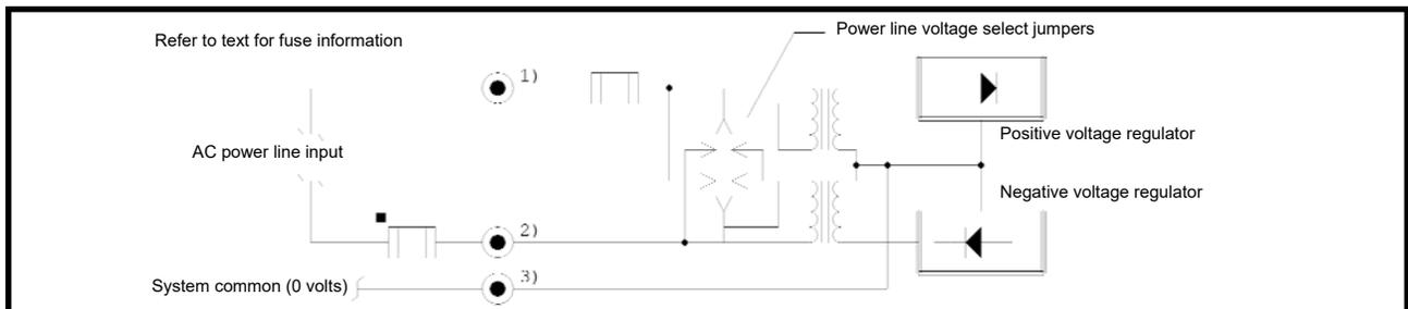
The external fuse shown in series with the connection to terminal number 2 should *not be installed* if this line is connected to the system earth ground.
