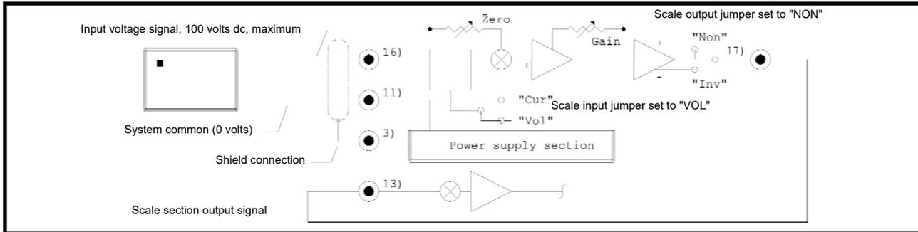
The figure above illustrates the connections required for both unidirectional and bidirectional operation with the command signal generated from a 100 volt (maximum) DC source. The output speed will increase in the forward direction as the input voltage is made more positive. A negative going increase in the input voltage will cause the output speed to increase in the reverse direction. With the input voltage command signal at zero volts the output will be stopped.
