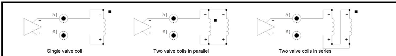
The pump displacement controller should be connected to the hydrostatic transmission controller in accordance with the drawing above. The polarity shown is with a positive input command signal. Signal current flow will be in the opposite direction when the input command signal is negative.
