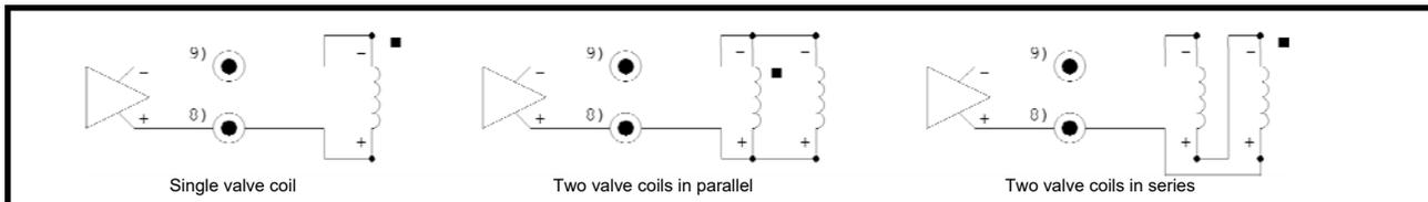
The motor displacement controller should be connected to the hydrostatic transmission controller in accordance with the drawing above. The polarity shown is with either a positive or negative input command signal. Signal current flow to the motor displacement controller is always in the direction shown.
