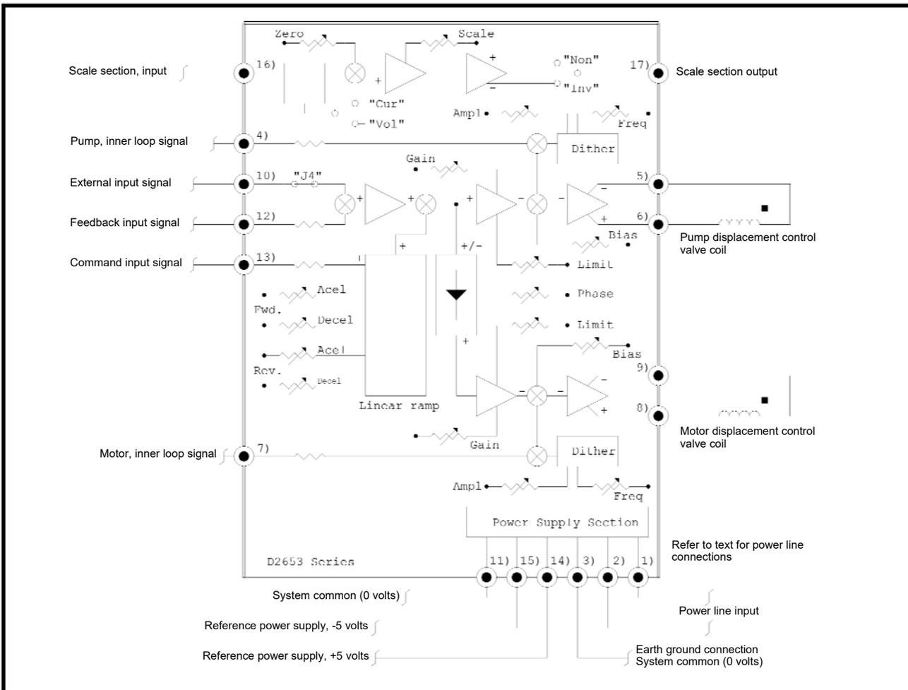
The functional drawing in the figure above illustrates the signal flow and polarity as well as the interconnections between the signal processing modules supplied on the hydrostatic transmission controller.
