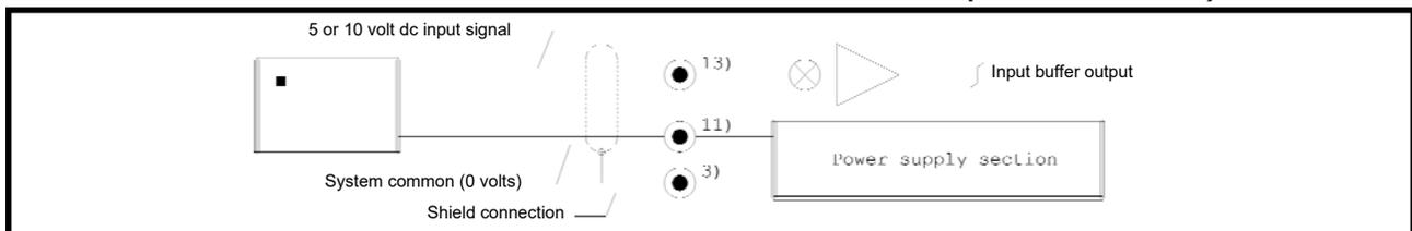
The figure above illustrates the connections required for both unidirectional and bidirectional operation with the command signal generated from a 5 or 10 volt DC source. The output speed will increase in the forward direction as the input voltage is made more positive. A negative going increase in the input voltage will
