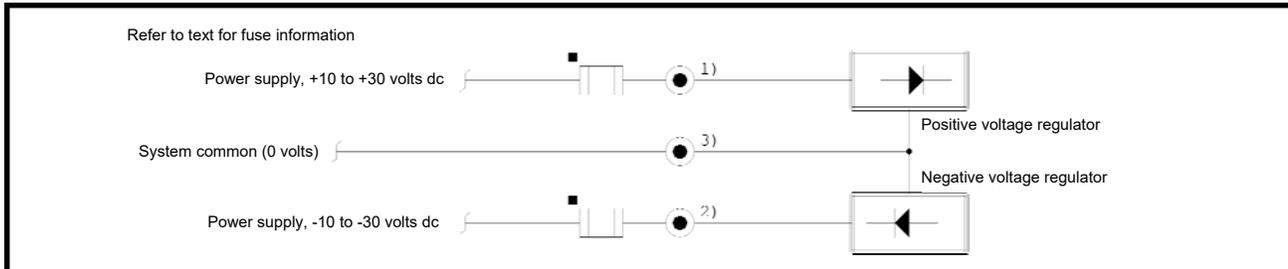
The fuses shown in the connections to terminal numbers 1 and 2 are not required if the user's external power supply includes the necessary short circuit protection devices.
