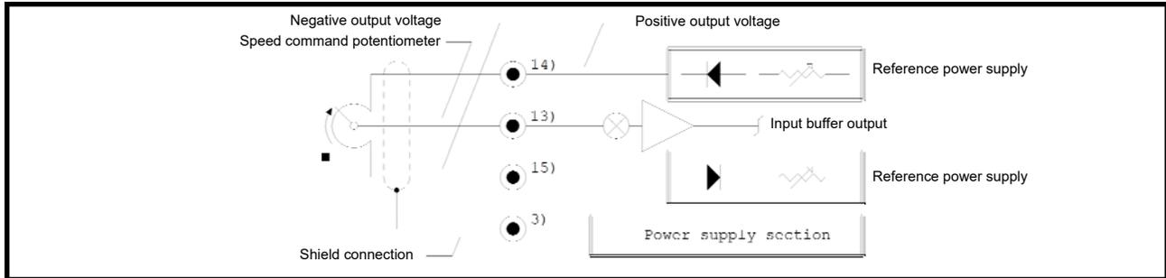
The figure above illustrates the connections between the external command potentiometer and the hydrostatic transmission controller to provide bidirectional (reversing) operation. The internal reference power supply is used to supply a bipolar command voltage. The "COMMAND INPUT" jumper should be placed in the "LO" position.
