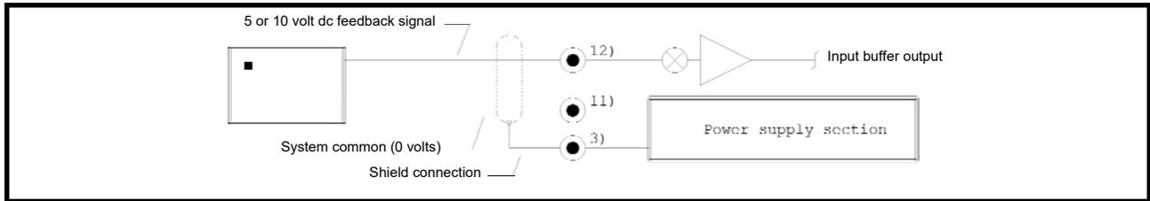
The figure above illustrates the connections required for both unidirectional and bidirectional operation with the velocity feedback signal generated from a 5 or 10 volt DC source.
