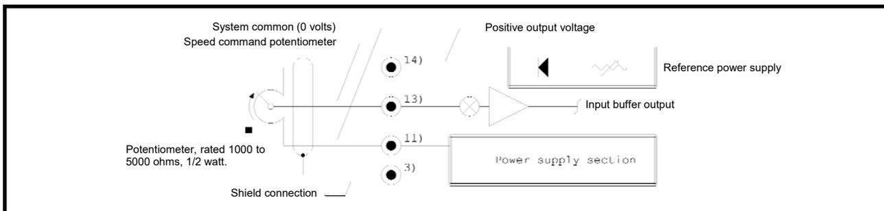
The figure above illustrates the connections between the external command potentiometer and the hydrostatic transmission controller to provide unidirectional (non-reversing) operation. The internal reference power supply is used to supply a positive command voltage. The "COMMAND INPUT" jumper should be placed in the "LO" position.
