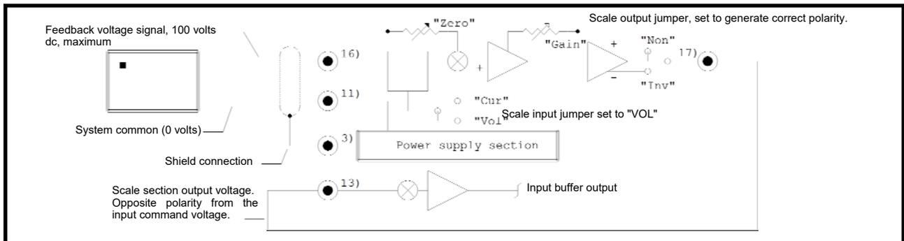
The figure above illustrates the connections required for both unidirectional and bidirectional operation with the command signal generated from a 100 volt (maximum) DC source.
