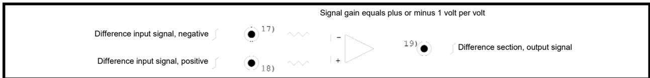
The output voltage signal from the difference amplifier section can be determined from the formula below:
