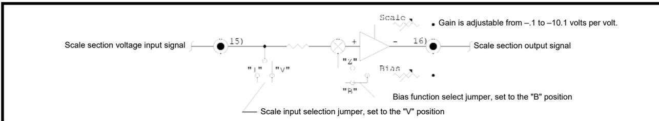
The output voltage signal from the scale section can be determined from the formula below:
