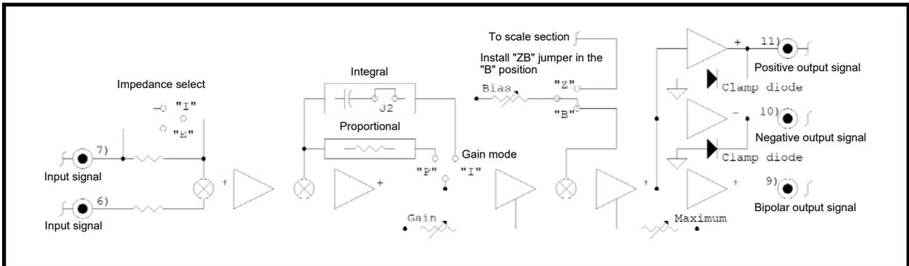
The clamp diodes shown on terminal numbers 10 and 11 will limit the negative signal on these terminals to approximately .3 volts DC
