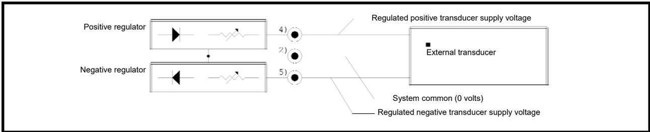
The transducer power supply output current is limited by the regulators ability to dissipate heat. The maximum output current at all ambient temperatures can be determined from the formula given below:
