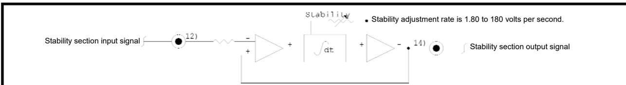
The stabilized voltage output signal on terminal number 14 will be of the same polarity and magnitude as the input signal on terminal number 12.
