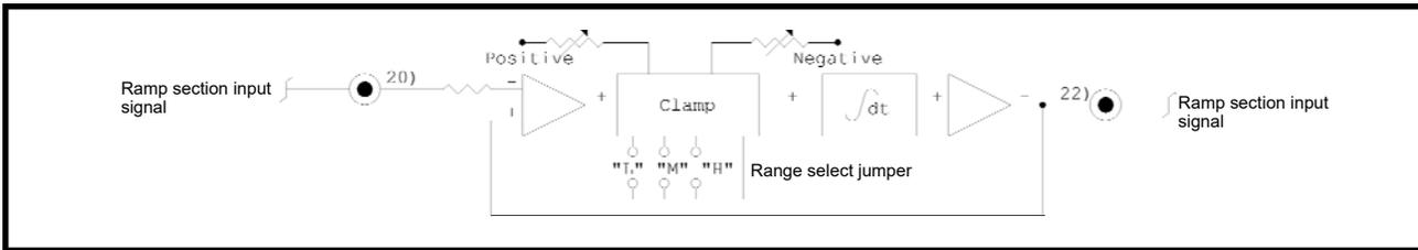
The stabilized voltage output signal on terminal number 22 will be of the same polarity and magnitude as the input signal on terminal number 20.
