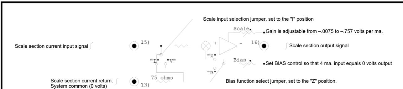
The output voltage signal from the scale section can be determined from the formula below:
