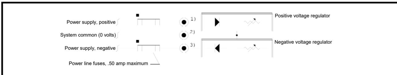
The fuses shown in the connections to terminal numbers 1 and 3 are not required if the user's external power supply includes the necessary short circuit protection devices.
