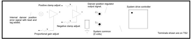
The output signal from the dancer position regulator will swing between the positive and negative clamp settings.
