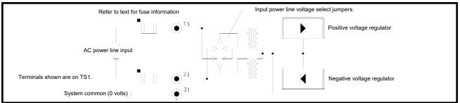
The external fuse shown in series with the connection to terminal number 2 on TS1 should *not be installed* if this line is connected to the system earth ground.
