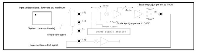
The figure above illustrates the connections required for both unidirectional and bidirectional operation with the command signal generated from a 100 volt (maximum) DC source. The output speed will increase in the forward direction as the input voltage is made more positive. A negative going increase in the input voltage will cause the output speed to increase in the reverse direction. With the input voltage command signal at zero volts the output will be stopped.
