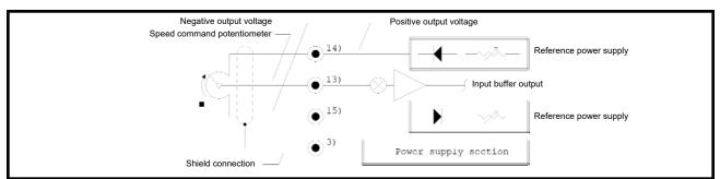
The figure above illustrates the connections between the external command potentiometer and the hydrostatic transmission controller to provide bidirectional (reversing) operation. The internal reference power supply is used to supply a bipolar command voltage. The "COMMAND INPUT" jumper should be placed in the "LO" position.
