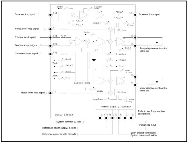
The functional drawing in the figure above illustrates the signal flow and polarity as well as the interconnections between the signal processing modules supplied on the hydrostatic transmission controller.
