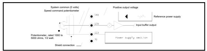
The figure above illustrates the connections between the external command potentiometer and the hydrostatic transmission controller to provide unidirectional (non-reversing) operation. The internal reference power supply is used to supply a positive command voltage. The "COMMAND INPUT" jumper should be placed in the "LO" position.
